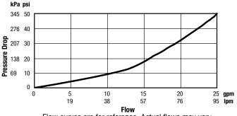
Flow curves are for reference. Actual flows may vary depending on system temperatures and/or pressures. \*\*\*Flow curve with integral inlet filters check valves
