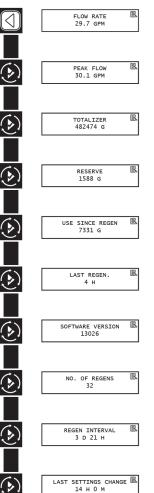
Peak flow since last regeneration Example: Gallons at the outlet since installation Example: Reserve Capacity setting
