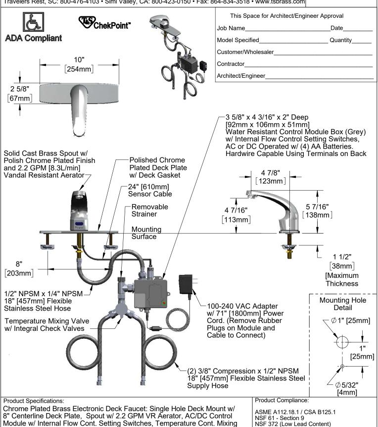
Valve w/ Integral Check Valves, 18" Hot & Cold Supply Stop Flexible
