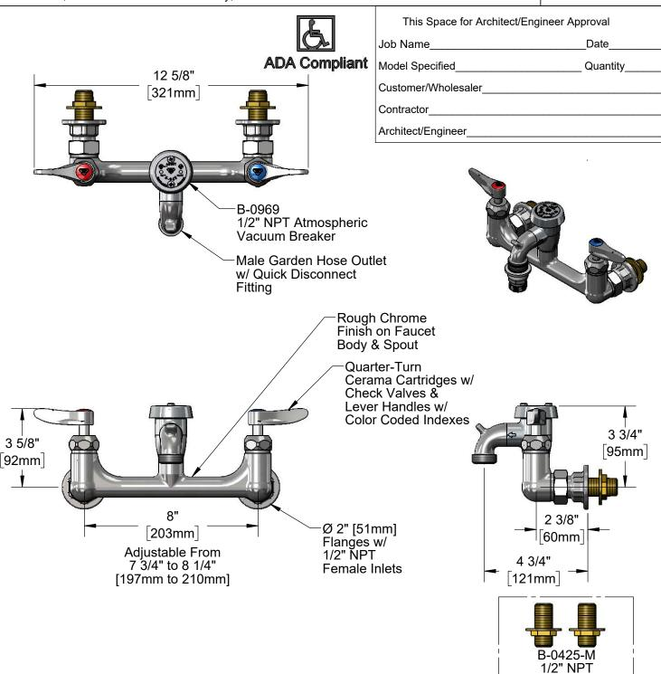
Rough-In Requirement: (2)  $\phi$  1" [25mm] Mounting Holes
