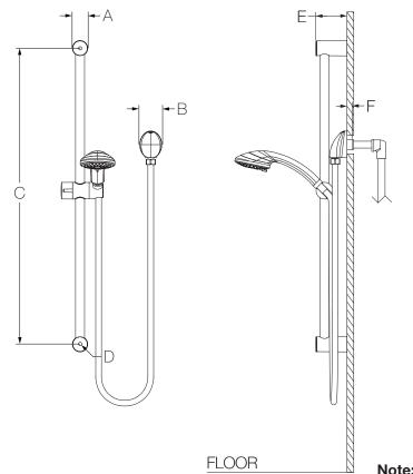
**Measurements** Ø 1-1/2", 38 mm А В 2-1/8", 54 mm 28-9/16", 725 mm С (2x) Hole Size: D Ø 1/4", 6 mm 3", 76 mm Е Male 1/2-14 NPT fitting must F be recessed 1/4" (6 mm) from finished wall
