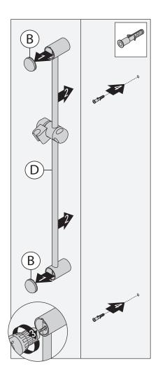
**Notes:** Make sure that slide bar holes and bracket holes are aligned before drilling. Before drilling bottom hole, make sure slide bar is plumb.
