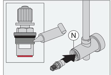
**Installation Tip:** Back off cartridge slightly to ensure proper handle alignment if necessary.
