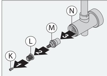
3) Apply removable thread lock to the threading of replacement cartridge. Install replacement cartridge into diverter body (N) at 50 in•lb.
