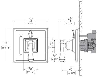
VALVE MOUNTING IS SHOWN FOR REFERENCE ONLY. VALVE IS NOT INCLUDED WITH CPT-8401-P
