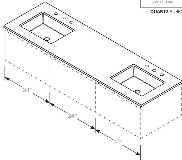
**Note:** Sinks must be located over H1-Tip Out or H2/V14 Plumbing drawers. See Cartesian Reference Guide for more information.
