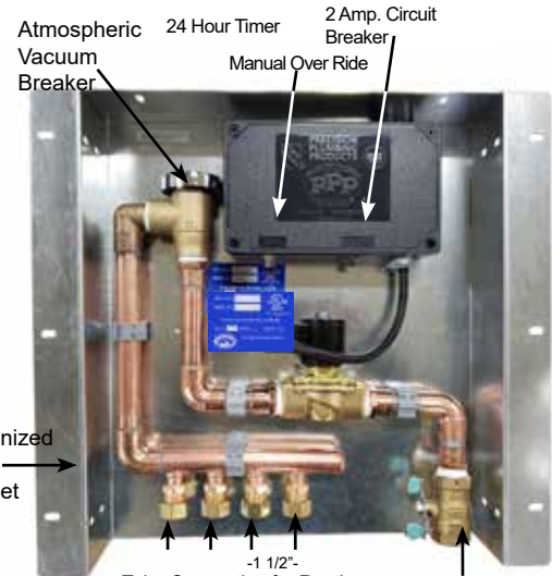
Special Calibrated Manifold for Equal Water Distribution to Floor Drains Tube Connection for Routing to Traps 1/2" / 5/8" Compression -1 1/2"- FNPT Water Source Connection Water On/Off Valve 3/4" FNPT Water Source Connection
