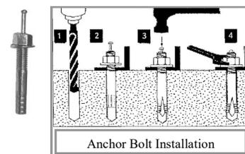
Anchor Bolt Installation
