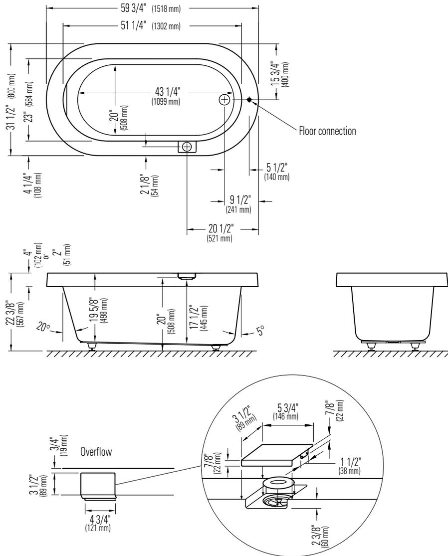
\*A bathtub fitted with back jets can cause the pump to protrude by approximately 3" from the overall dimension.
