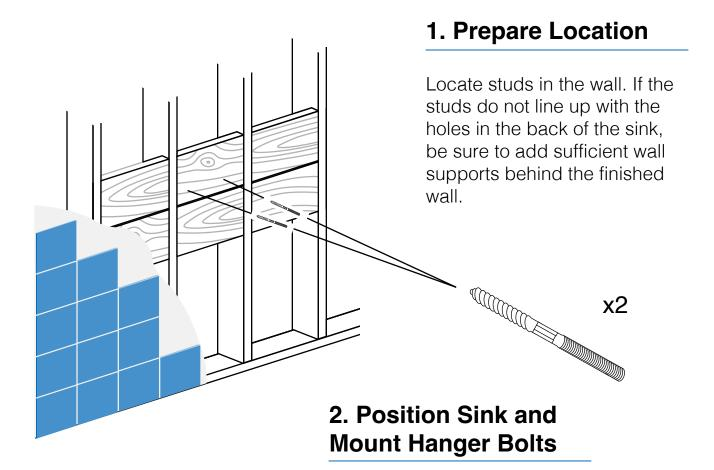
Position sink and mark the mounting hole locations. Drill pilot holes in wood and screw in hanger bolts. Check postion with a level.
