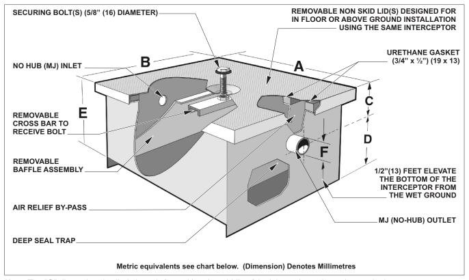
**Note:** The "C" dimension detailed above is from either the middle of the inlet or the outlet to the top the interceptor. The inlet and outlet dimensions are always the same.
