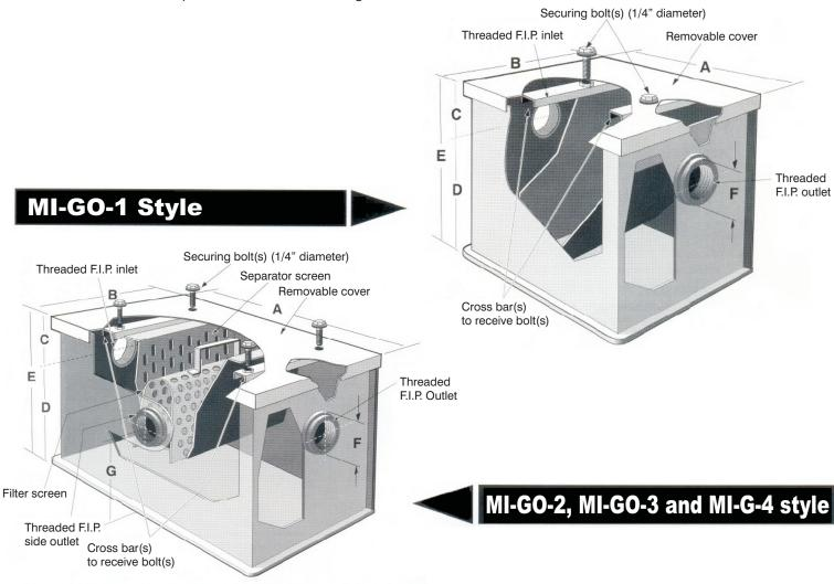
The separator screen is perforated at one end only. This end should always face the inlet. The separator screen can be reversed to change the inlet location. The MI-GO-2 style has a male threaded side outlet. The MI-GO-3 and MI-GO-4 style has a female threaded side outlet. THE MI-GO-3 and MI-GO-4 style have 4 bolts securing the lid to the body. The MI-GO-2 style has 2 bolts securing the lid to the body.
