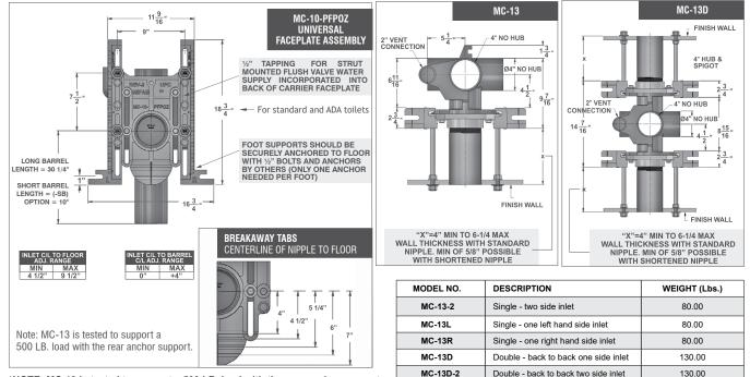
\*NOTE: MC-13 is tested to support a 500 LB. load with the rear anchor support.
