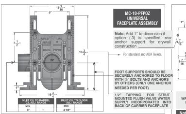
\*MC-10 is tested to support a 500 lb. load with the rear anchor support.
