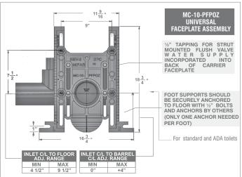
\*MC-10-27 is tested to support a 500 lb. load with the rear anchor support.
