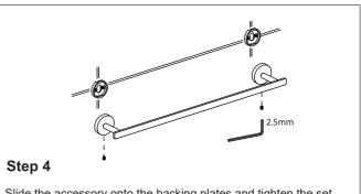
Slide the accessory onto the backing plates and tighten the set screws using Allen key provided.
