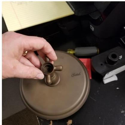
8. Set #7 washer into center of #10 cross handle and thread #6 slotted handle screw into cross handle tightly with slotted screwdriver.
