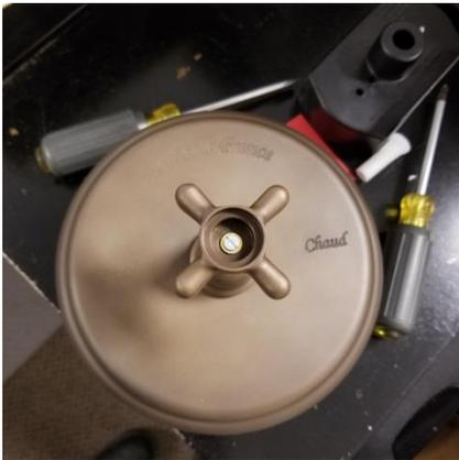
9. Take #91 logo insert and apply a small amount of plumber's grease to the rubber o-rings on the plug. Align correctly and insert the logo plug into the center of the cross handle:
