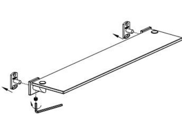
② ALIGN MOUNTING BRACKETS AND MARK LOCATION
