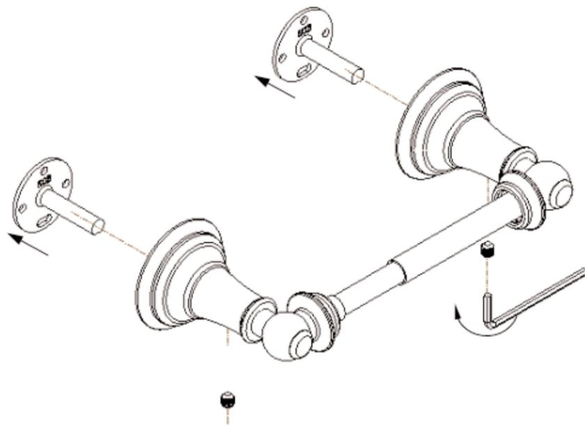
② ALIGN MOUNTING BRACKETS AND MARK LOCATION
