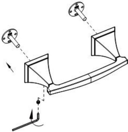
② ALIGN MOUNTING BRACKETS AND MARK LOCATION
