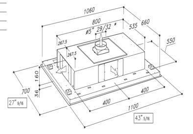
\* accessory outlet Ø8" For the installation, create a false ceiling with a niche of 1065mm for 665mm whose minimum height to be reached is 270mm
