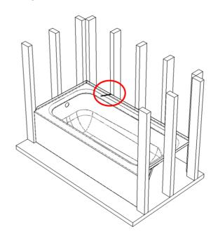
7. Measure tile flange height and mark distance from top marking on studs
