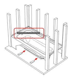
6. Install tub and mark top of tile flange with pen
