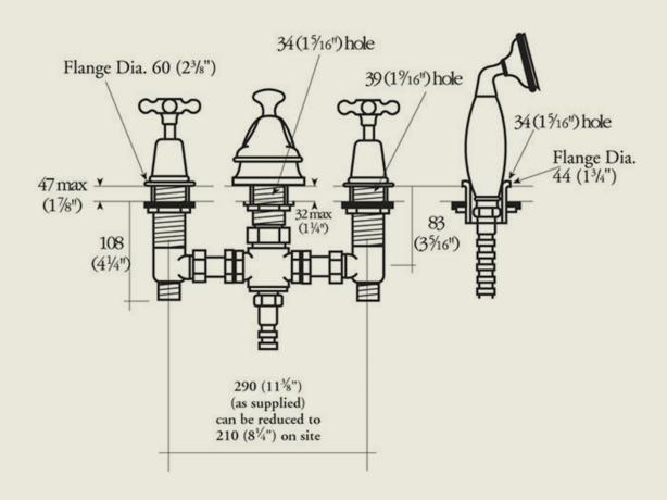
Model No. R3484-1900 Internals Standard-3/4 ceramic cartridge Optional compression cartridge available
