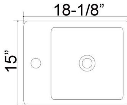
Dimensions of fixture are nominal and may vary within the range of tolerances established by ASME Standard A112.19.2.2013 Dimensions and specifications subject to change without notice.
