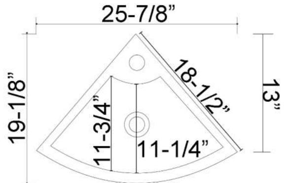
Dimensions of fixture are nominal and may vary within the range of tolerances established by ANSI Standard A112.19.2.2018. Dimensions and specifications subject to change without notice.
