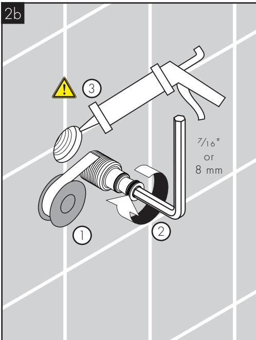
Wrap the mounting piece with plumbers' tape. Install the mounting piece.
