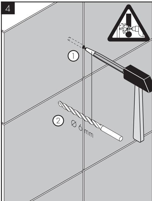
Mark and drill a hole using a  $\frac{1}{4}$ " (6mm) drill bit appropriate for your wall surface.
