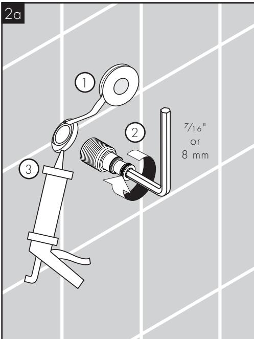
Wrap the threads on the nipple with plumbers' tape. Install the mounting piece.
