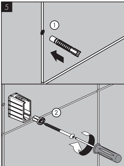
Insert the provided anchor, and then install the bracket using the provided eccentric bushing and screw
