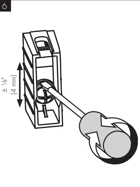
The eccentric bushing allows adjustment of approximately  $\frac{1}{8}''$  (4 mm) up and down
