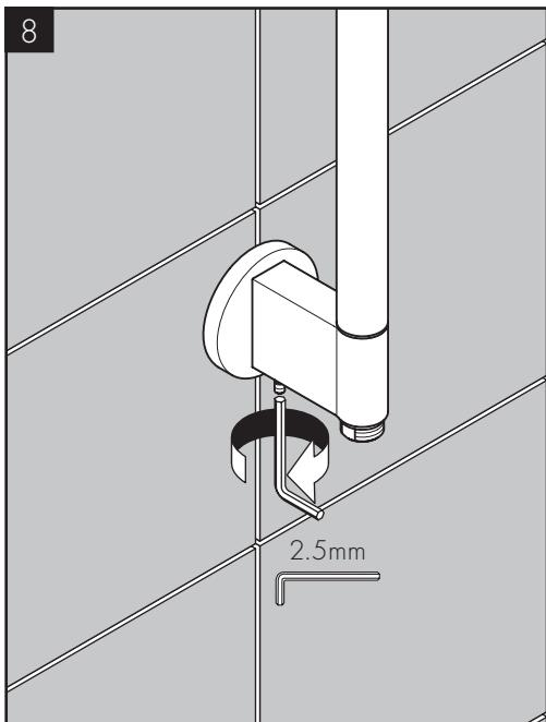
Tighten the setscrew at the bottom of the wallbar assembly using a 2.5 mm allen wrench.
