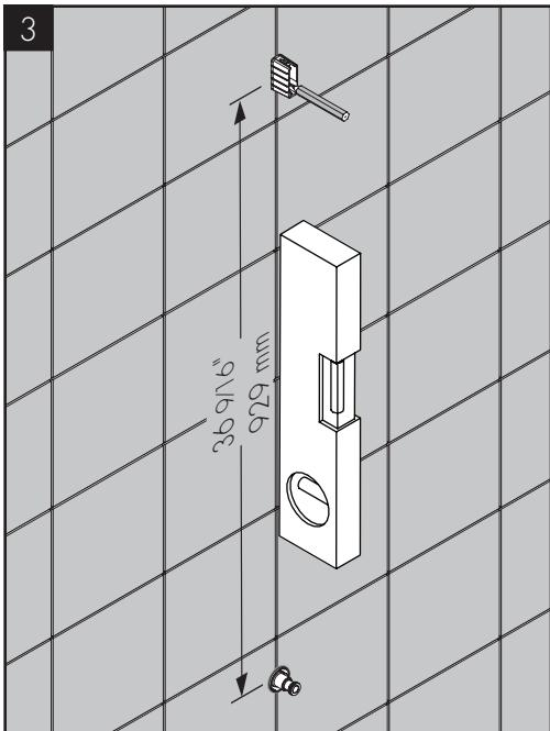
From the center of the mounting piece, measure  $36 \frac{9}{16}$ " (929 mm) up the wall. Make sure that the line is level.
