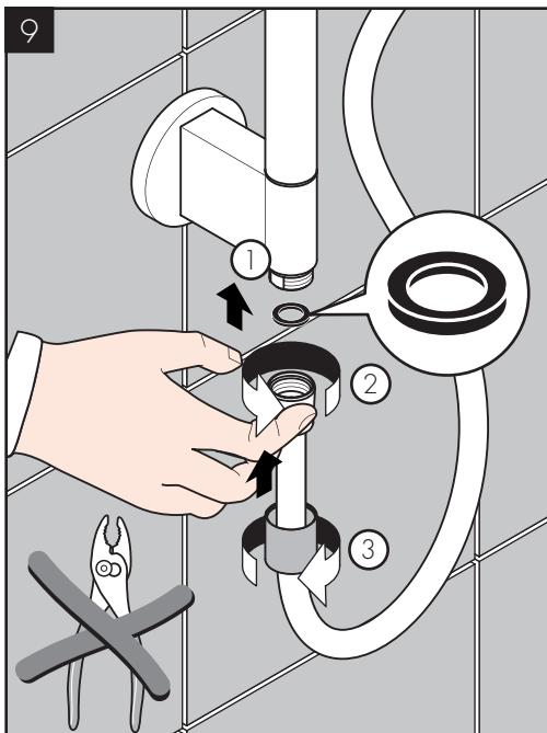
Connect the hose to the wallbar assembly using a hose washer
