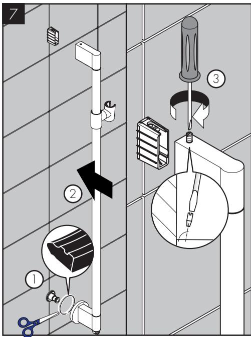
Install the foam seal in the escutcheon as shown, with the narrow side facing the wall. Trim the seal if it is too long.
