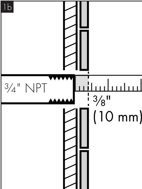
This installation requires a  $\frac{3}{4}$ " NPT female threaded pipe fitting recessed  $\frac{3}{8}$ " (10 mm) behind surface of finished wall.
