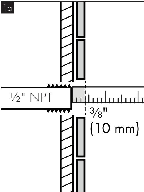
This installation requires a  $\frac{1}{2}$ " NPT male nipple recessed  $\frac{3}{8}$ " (10 mm) behind surface of finished wall.
