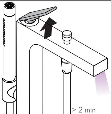
Flush the hot and cold supply lines for at least two minutes.
