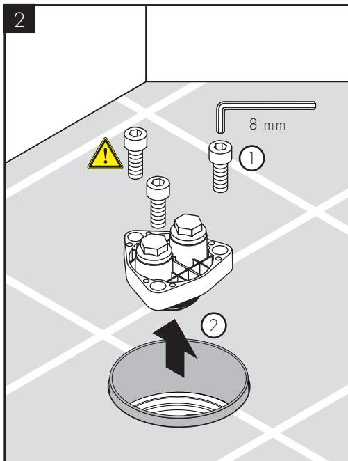
Remove the flush housing screws.
