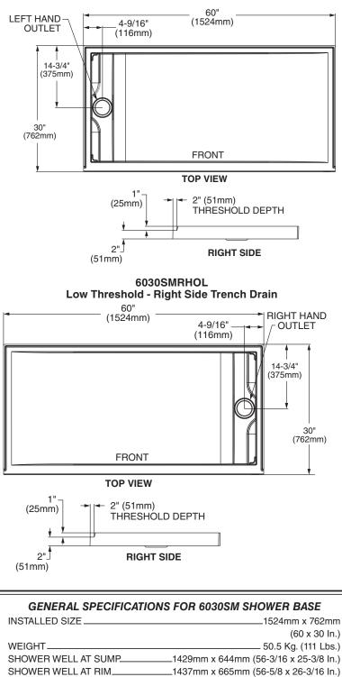
6030SMLHOL Low Threshold - Left Side Trench Drain
